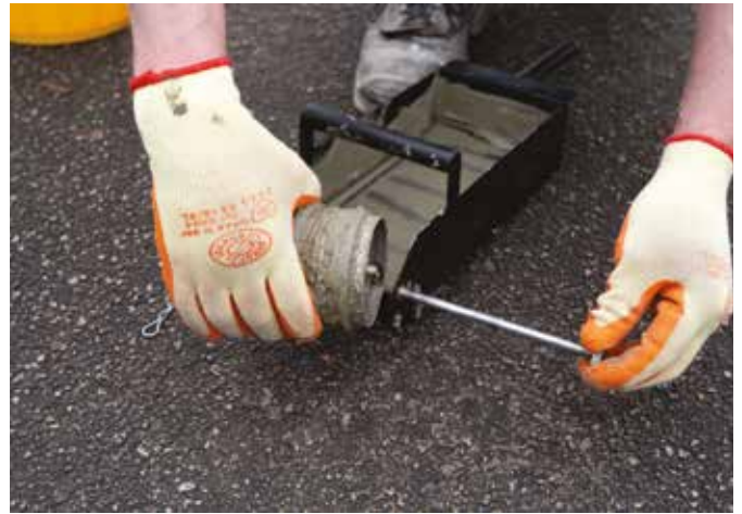
2. When you're done with the roller, simply remove the split pin & spindle to release the drum.
