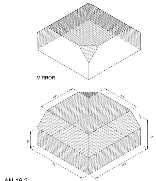
AN.16.2 DOUBLE CANT EXTERNAL RETURN WITH INTERNAL SLOPE (SCOB)
