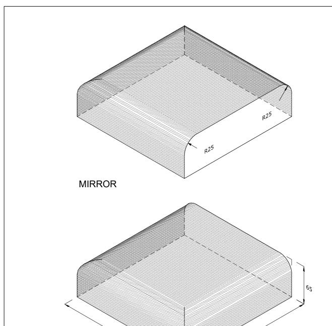
BN.15.7 STOP END TO DOUBLE BULLNOSE ON EDGE AND TO BULLNOSE DOUBLE HEADER ON FLAT (SCOB)
