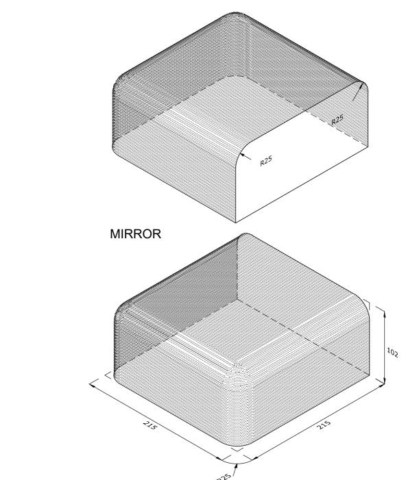
BN.18.3 STOP END TO DOUBLE BULLNOSE ON EDGE AND TO BULLNOSE DOUBLE HEADER ON FLAT (RCOB)
