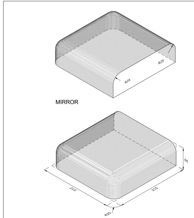
BN.18.7 STOP END TO DOUBLE BULLNOSE ON EDGE AND TO BULLNOSE DOUBLE HEADER ON FLAT (RCOB)
