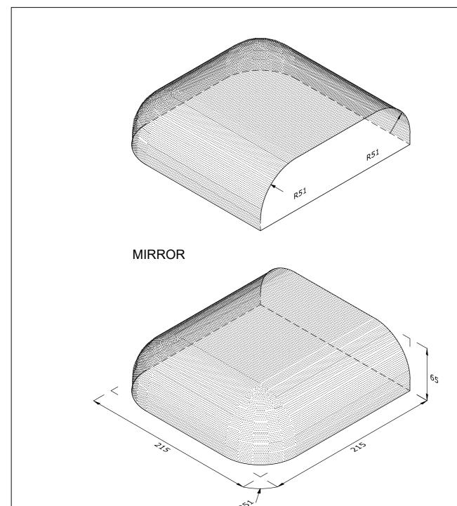
BN.18.8 STOP END TO DOUBLE BULLNOSE ON EDGE AND TO BULLNOSE DOUBLE HEADER ON FLAT (RCOB)
